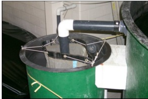
Figure 2. Egg collection utilising an external collection tank. The bag is connected to the outflow pipe of the broodstock tank (Photo courtesy of The Ocean Sciences Centre, Newfoundland).
