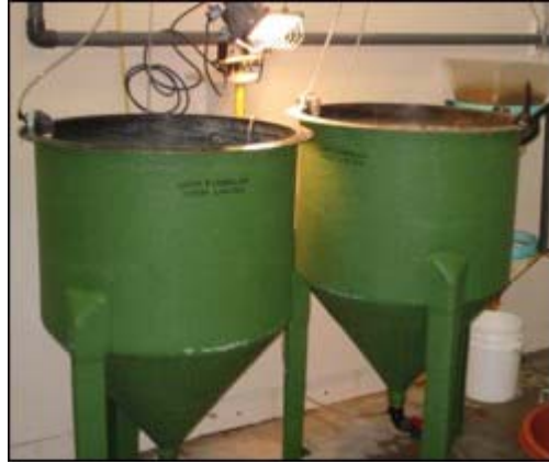
Figure 6. Artemia production tanks. A “decapsulation cone” can be seen at the far right. Dehydrated cysts, purchased from a supplier, have to be decapsulated before the hatching process can begin. Artemia grow and receive enrichment in these tanks before being transferred to the larval tanks. (Photo courtesy of The Ocean Sciences Centre, Newfoundland).
